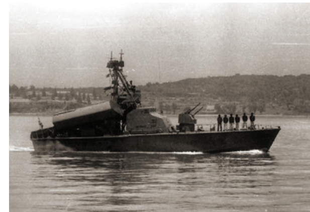
Russian-manufactured missile boat armed with Styx ship-to-ship missiles (note large missile launcher toward the rear of the ship angled upward).
